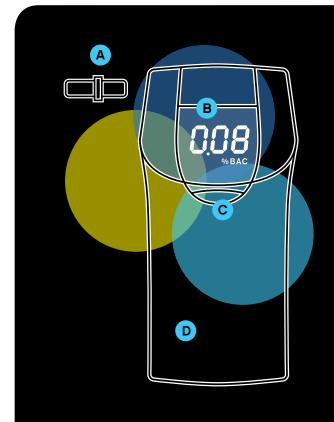
A Replaceable, hygienic mouthpiece provides a safe and sanitary method for testing multiple users
