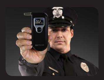
The latest addition to the BACTRACK Breathalyzer Series, the BACTRACK B90 is a professional breath alcohol tester designed for use by law enforcement, hospitals, businesses, and even for consumer use. The BACTRACK quickly and easily estimates BAC - blood alcohol content - based on a deep lung air sample. Simply activate the FlipBlade™ mouthpiece and begin testing in seconds. The BACTRACK B90 is accurate enough for professional use yet simple and safe enough for anyone to operate.
